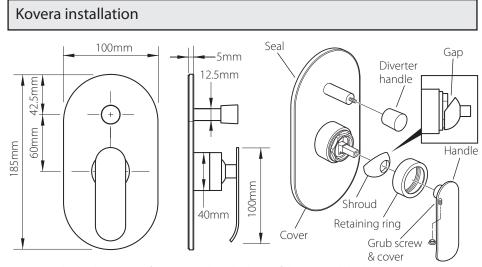
Remove the backing paper from the seal on the back of the cover. Slide the cover over the valve, push onto the wall until it makes contact.
