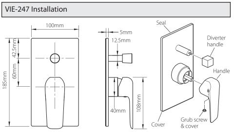
Remove the backing paper from the seal on the back of the cover. Slide the cover over the valve, push onto the wall until it makes contact.
