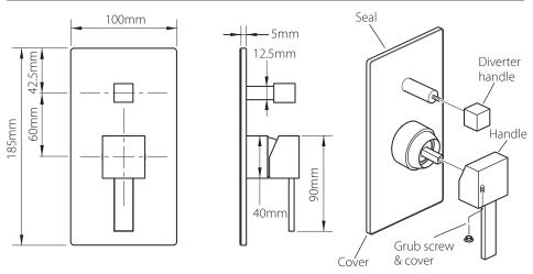
Remove the backing paper from the seal on the back of the cover. Slide the cover over the valve, push onto the wall until it makes contact.
