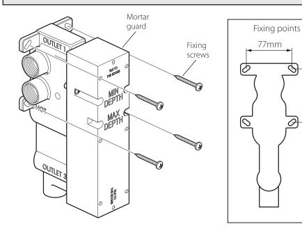
Select the position for the shower valve and offer the shower valve to the wall, make sure the valve is vertical with a level and mark the 4 fixing points with a suitable pencil, see above right for dimensions. Remove the shower valve from the wall, drill the holes to a suitable depth for the wall plugs and secure with suitable screws.
