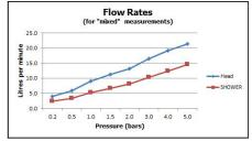
'mixed measurements' refers to equal hot and cold water supply flow rate for unregulated flow unless flow regulator fitted as standard
