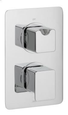
**DESCRIPTION:** DX Phase concealed 1 outlet, 2 handle thermostatic shower valve wall mounted with rectangular backplate thermostatic cartridge V-001C-PLA flow cartridge C-301-RTC 2 x 3/4" female inlets 1 x 3/4" female outlet includes 3/4" - 1/2" adaptors inc. bleed valve for system flush on installation min-max wall mount 70-95mm optimum installation depth 82mm minimum operating pressure 0.2 bar LP (shower) minimum operating pressure 1.0 bar MP (bath)
