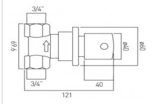
concealed stop valve 3/4" wall mounted ceramic cartridge ELE-VALVE/CD-3/4 1 x 3/4" female inlet 1 x description:
