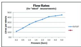
'mixed measurements' refers to equal hot and cold water supply flow rate for unregulated flow unless flow regulator fitted as standard
