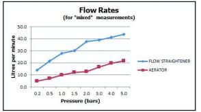
'imixed measurements' refers to equal hot and cold water supply flow rate for unregulated flow unless flow regulator fitted as standard
